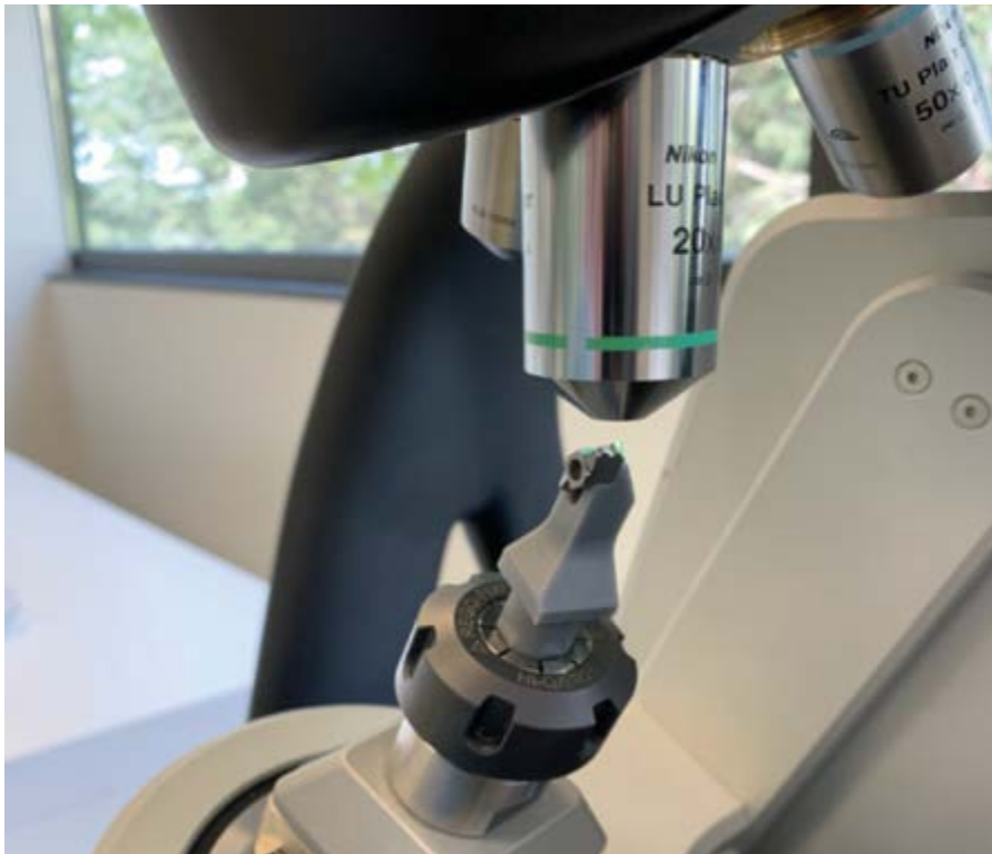
Figure 3. Positioning of the insert under the S neox Five Axis 3D optical profiler.
