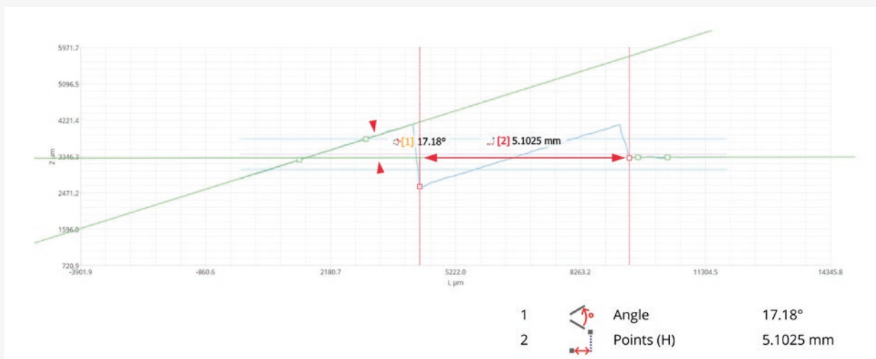
Figure 3. Close-up view of the insert and critical dimensions taken from the profile view.
