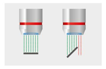
The inclination of a sample significantly affects the measured roughness, as the sampling changes with different inclinations.
