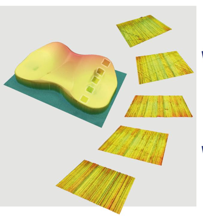
When measuring roughness on a tilted sample, the results can be useful if used qualitatively—for example, when comparing different implants measured in the same region. However, these measurements are not quantitatively accurate for the following reasons.
